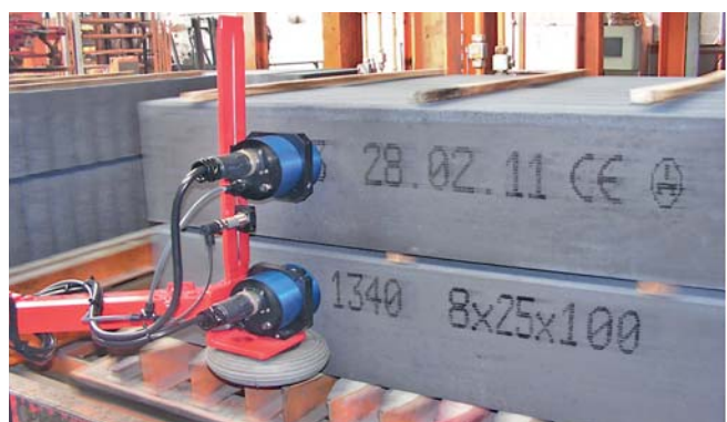
Coding of precast concrete elements
