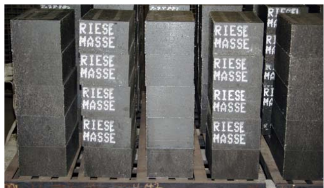
Refractory stone marking with high-temperature ink
