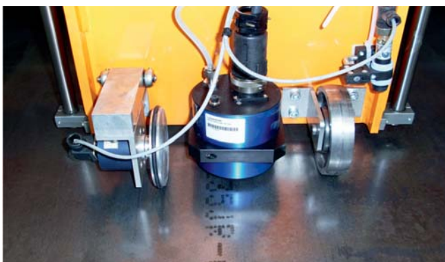
Steel sheet marking with etching ink
