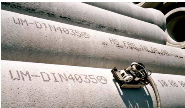
Mobile marking of concrete pipes
